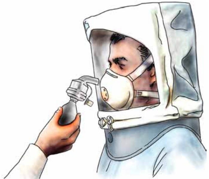
Fit testing for a disposable respirator using a special hood
